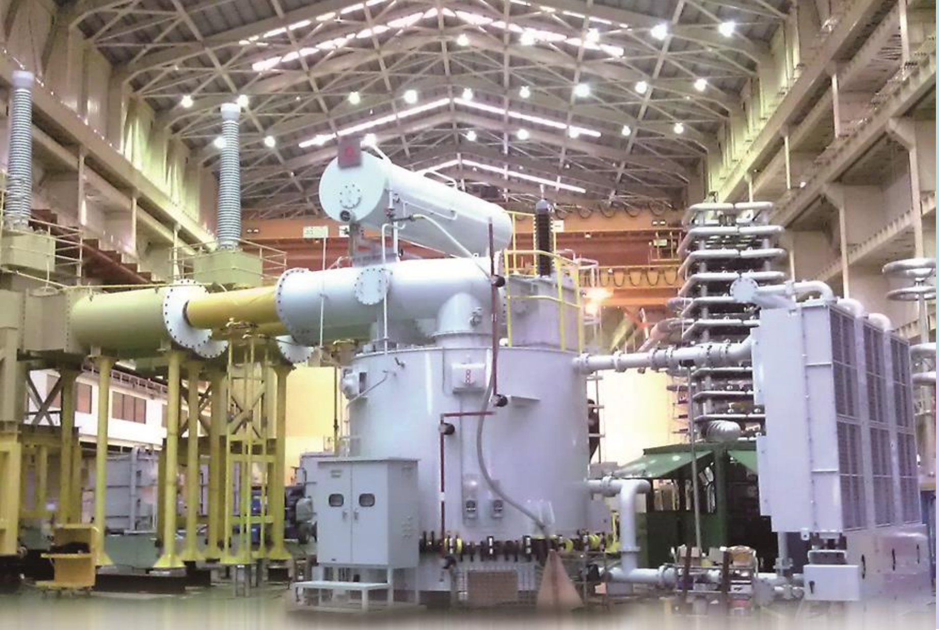
TAIWAN's First and Largest Capacity Shunt Reactor " 345 kV 100MVAR "
