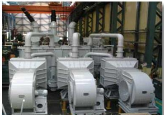
SF 6 Gas-Insulated Transformer 161kV-60MVA
